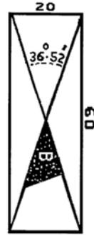
Laying a 1x3 Rectangle using the Larger Acute Angle of the 3-4-5 Triangle
