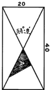
Laying a 1x2 Rectangle using the Larger Acute Angle of the 3-4-5 Triangle
